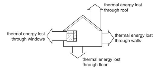
The heating system must supply more than 54 MJ of thermal energy to keep the temperature of the house constant.
