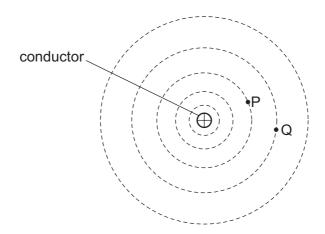
The current in the conductor is into the plane of the diagram.
